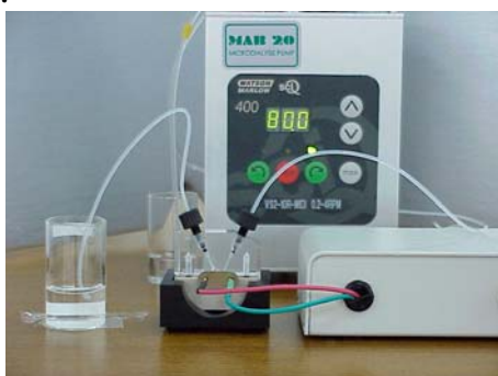
Fig. 5 a FI-QCM detection
